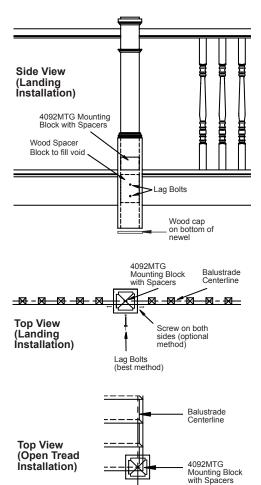
8. Coat the mounting block assembly with construction adhesive. Set the newel over the assembly and secure it to the mounting block assembly using an appropriate mounting method. Secure the newel to the face of the balcony by using lag bolts installed through the face of the newel. Screws may also be installed through the sides into the face of the plywood spacer block. Plug and sand all holes.
